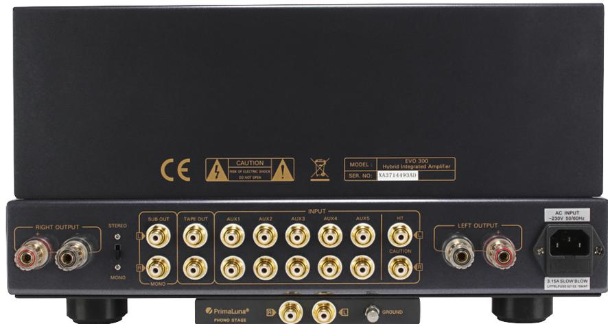
**At rear a line of solid, gold plated phono input sockets, one pair of speaker sockets and – beneath – casework for an optional MM phono stage. Above lies the power amplifier with its 500VA mains transformer.**
